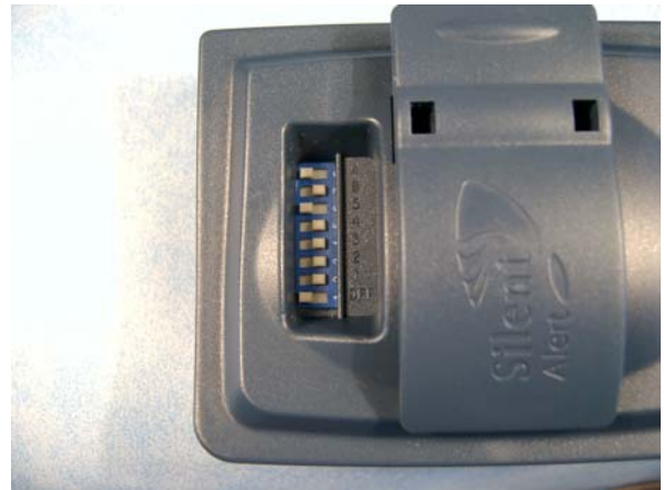
Pager back showing key switches
